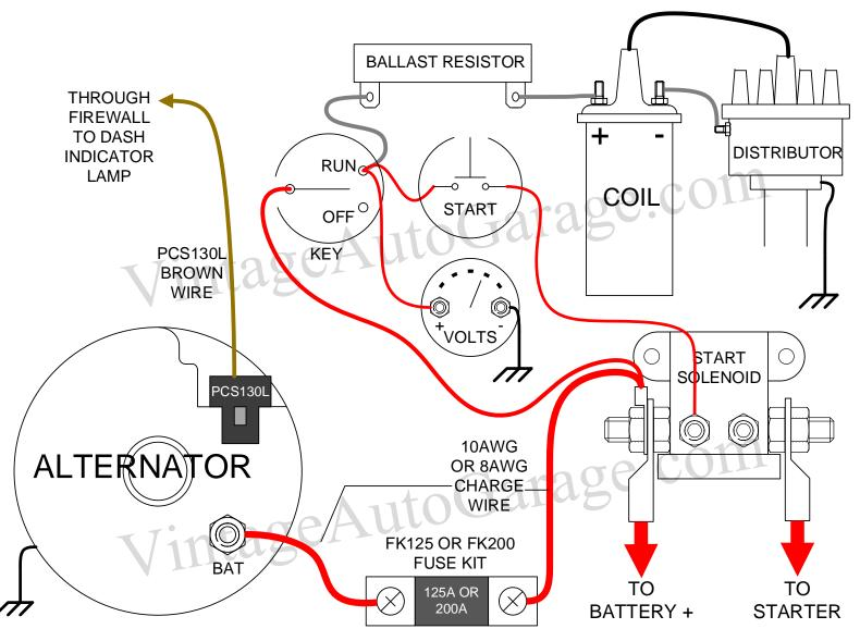
Connections shown are typical. Your installation may differ depending on components in your system, such as with a foot pedal starter system without start button, or switched ground control of starter solenoid.
